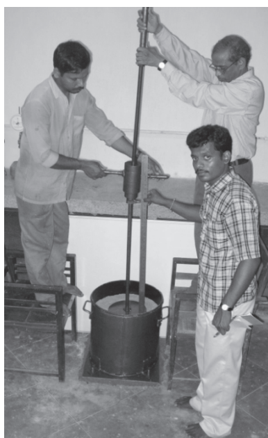
Fig.5 Test Box for Conducting DCP Tests
